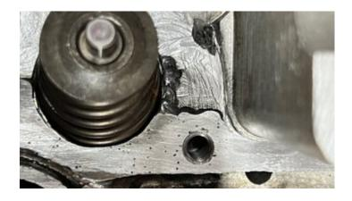
The background is: Cylinder heads in Porsche vehicles are often destroyed by cracking as a result of excessive heat input. This results in further engine damage. We notice this again and again in connection with engine repairs.
