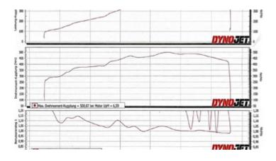
A power measurement on a <u>#roller</u> <u>#dynamometer</u> <u>#measures</u> the power that is <u>#transferred</u> from the <u>#wheels</u> to the rollers.
