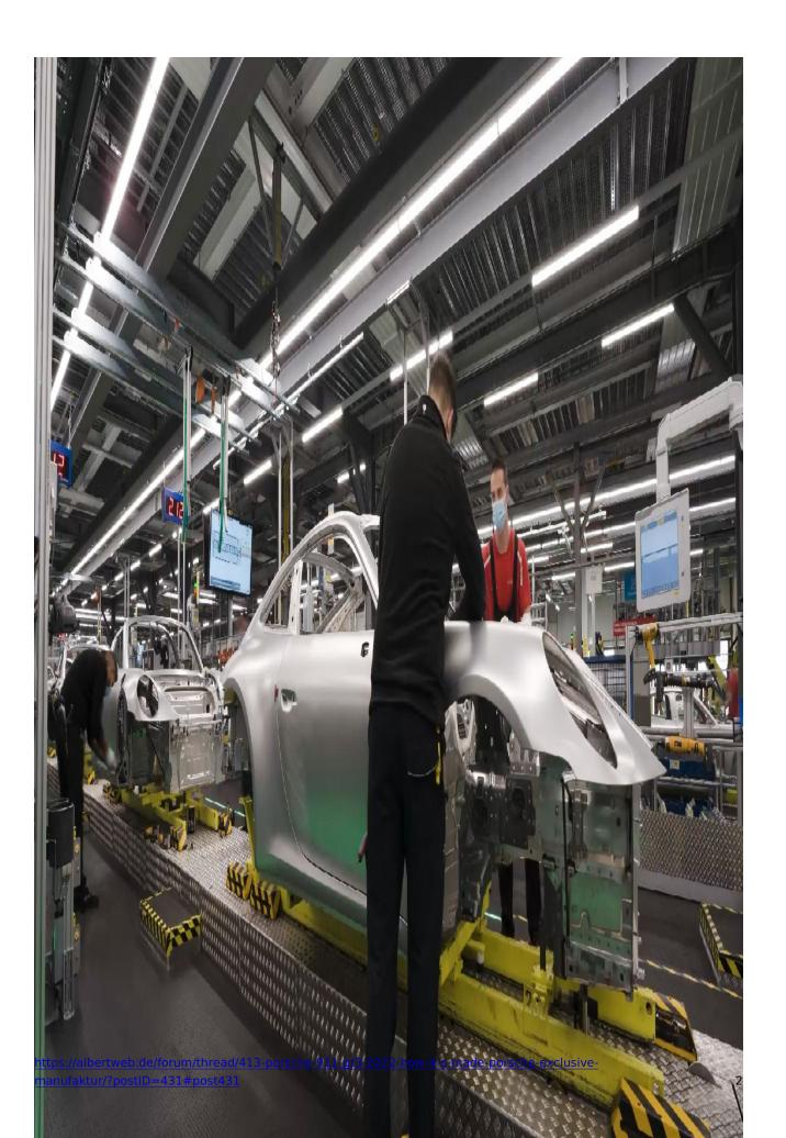
Prior to its 117-stage assembly, the 911 chassis has spent more than a day going through preparation in the body and paint shop. One of the challenges of painting vehicles and developing paint finishes is working with the material mix of the underlying components. A vehicle body already consists of several different steel and aluminum materials and can also include carbon fiber or polypropylene. Paint batches must suit all exterior features equally and produce the same color.
