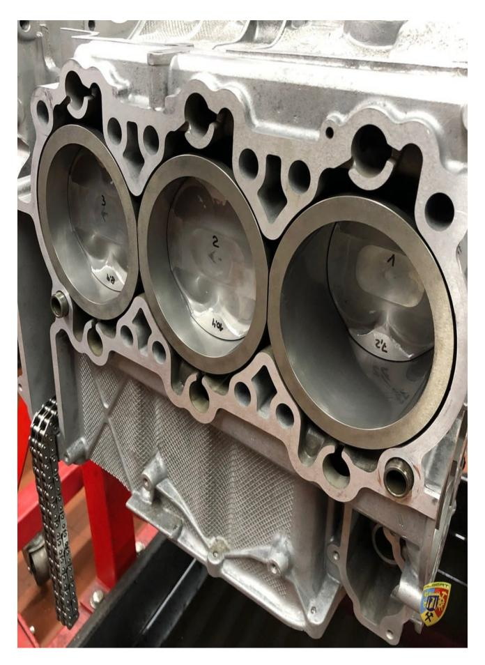
We completely eliminate the unstable Porsche cylinders and install completely new, solid graphite cylinders.
