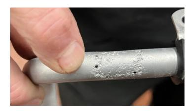
The lines are made of bare aluminum and very often have severe pitting. This pitting, a form of corrosion, takes place just below the rubber-protected sheet metal brackets.
