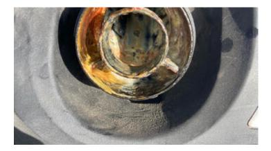
What is that <u>#sludge</u> in the oil and where does this sludge in the oil cap come from?
