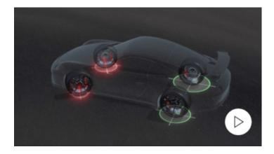
If our Porsche has too little grip on the #front axle and thus steers less into the #curve than the steering wheel specifies, then it understeers and pushes into the curve via the front wheels.
