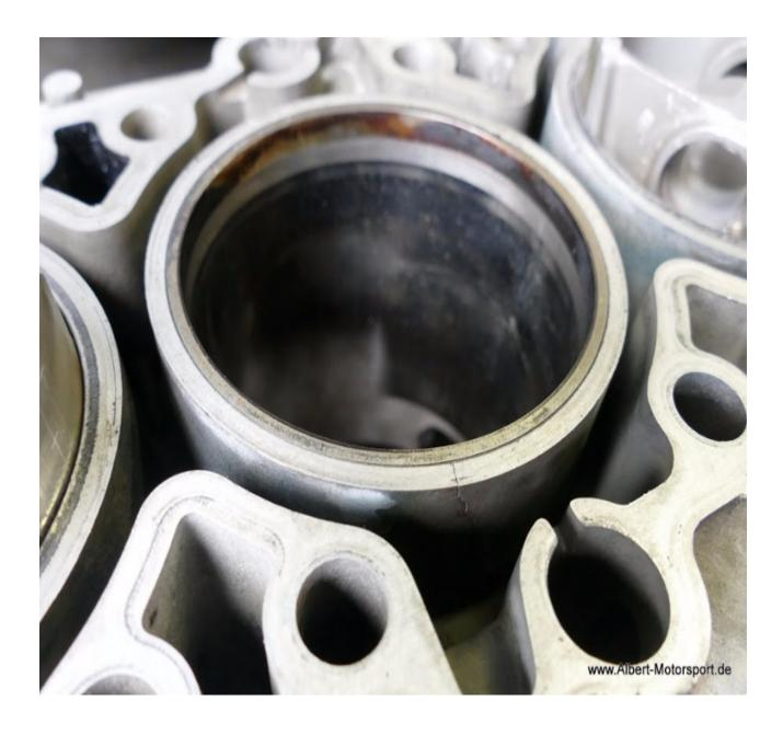
With different materials: Corrosion formation, gap formation, water penetration, leaks, cracks, engine damage.
