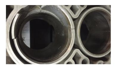
Then suddenly, usually when driving on the highway, there is a powerful knock or a very strong clicking from the engine with a subsequent blockage of the engine.
