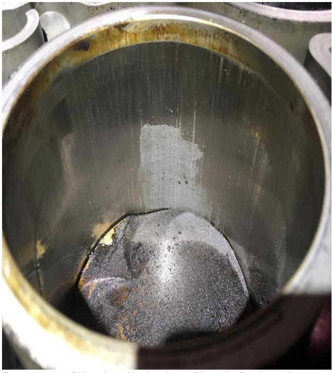
The consequences of this are in coatings. Detachment of the coating from the metal.
